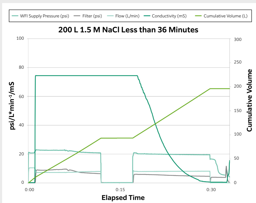
Figure 1. Batch record for the hydration of 200 L of 1.5 M Sodium Chloride. Preparation of 200 L of 1.5 M Sodium Chloride was performed using the Oceo Rover resulting in a total hydration time of approximately 35 minutes.
